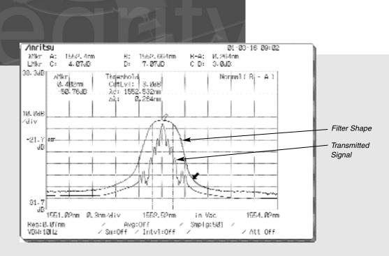
It can be seen from the diagram above that as the channel spacing gets closer, the shape of the filter becomes more critical. *Extracting a 10-Gbps signal when channels are spaced at 50-GHz, is technically difficult.*
