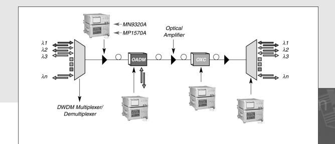
When we consider that these adjacent channels may only be 0.4 nm or 50-GHz apart from one another, the slightest change in a neighboring characteristic may lead to significant data transmission errors in another channel.
